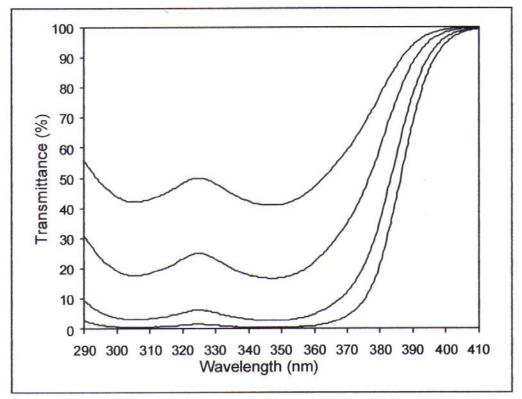
Top line: 0.001% ADA1160, corresponds to 0.25% in a 40  $\mu m$  film. Second line: 0.002% ADA1160, corresponds to 0.50% in a 40  $\mu m$  film. Third line: 0.004% ADA1160, corresponds to 1.0% in a 40  $\mu m$  film. **Bottom line:** 0.006% ADA1160, corresponds to 1.5% in a 40  $\mu m$  film.
